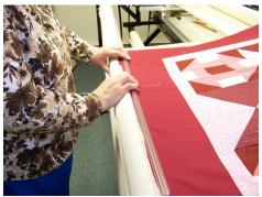
Be aware that there will be a small bump on the roller as you roll it. If it hinders the movement of the machine, adjust the height of the roller. Most times as you roll it, it will not be a problem.
