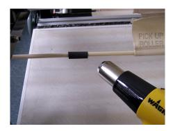
Allow to cool for a couple of minutes, then repeat steps 1 & 2 to join the third section to the second rod. Repeat for the other two leaders. If you float your top, you won't need to do the top leader. Make sure all the fabric is being gripped. Check the clear plastic to see that the fabric edge is just past the grip edge, about 1/8 of an inch. Slide end mini grips out of the way as you come to them.
