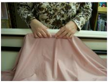
Make sure all the fabric is being gripped. Check the clear plastic to see that the fabric edge is just past the grip edge, about 1/8 of an inch. Slide end mini grips out of the way as you come to them.
